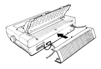
**Note:** The cable cover should always be attached when you use the printer.
